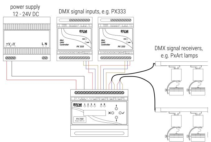
**NOTE!** DMX 1 and DMX 2 are always signal inputs. DMX 3, depending on the merge mode, can be the output (2/2) or the input (3/1) of the DMX signal. DMX 4 is always the output.
